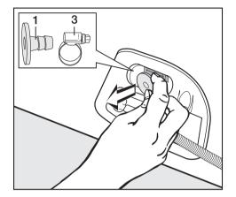
Remove the following from the back of the dryer at the bottom:
